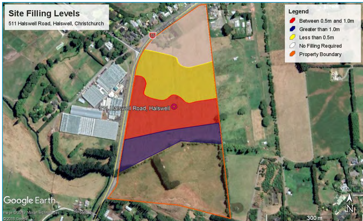
Figure 6: Approximate extents of Site Filling
