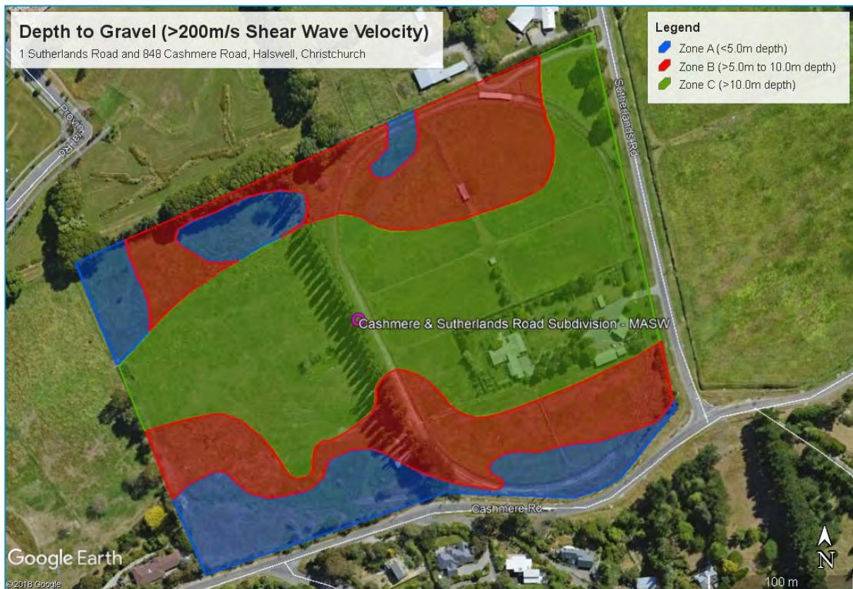
Figure 4: Depth to Gravel based on MASW Survey Results
