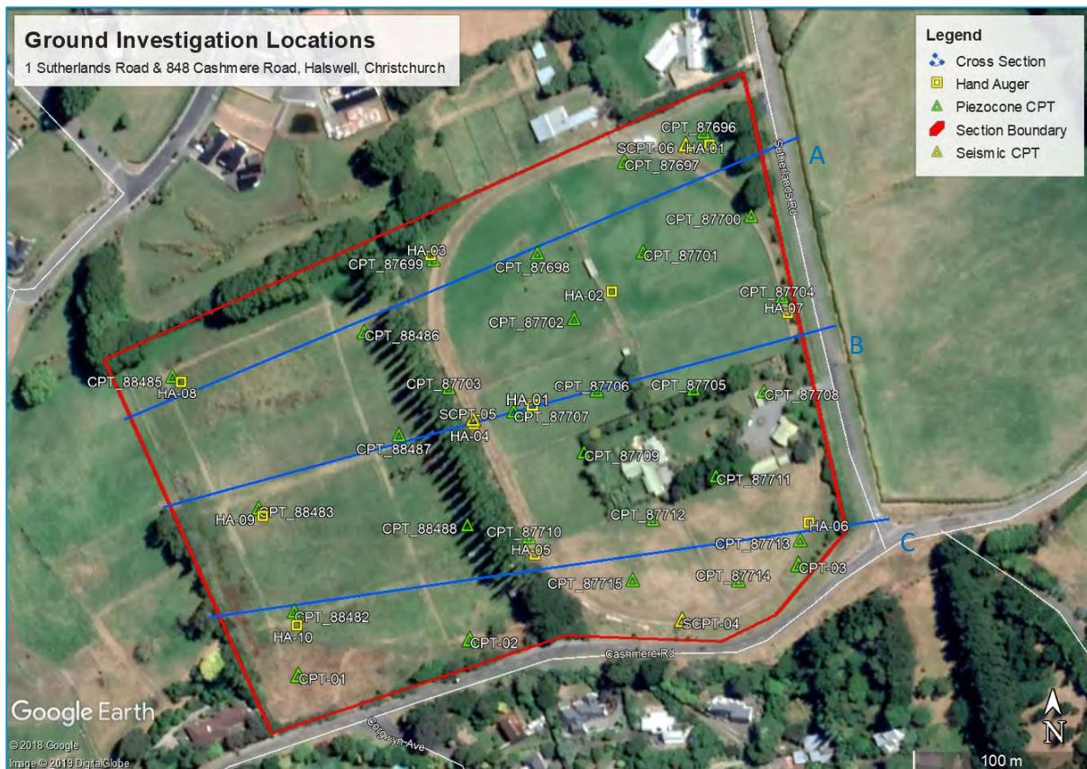
Figure 2: Site Investigation Location Plan (Scale as Shown)
