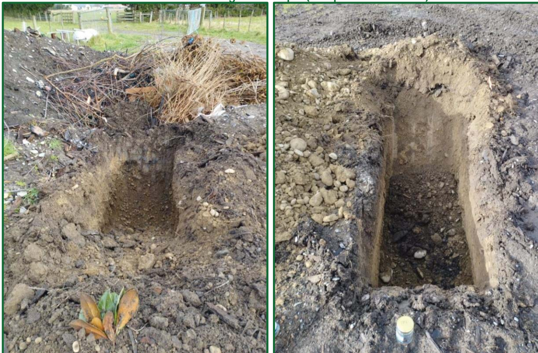
Photo 3 & 4 – Test pit within existing rubbish pit (sample location TP1)
